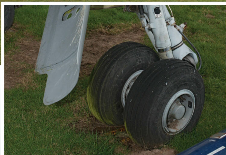
The landing gear's low-pressure tyres retract into the fuselage on takeoff. The IAF initially reported failures, which led to the system being upgraded
